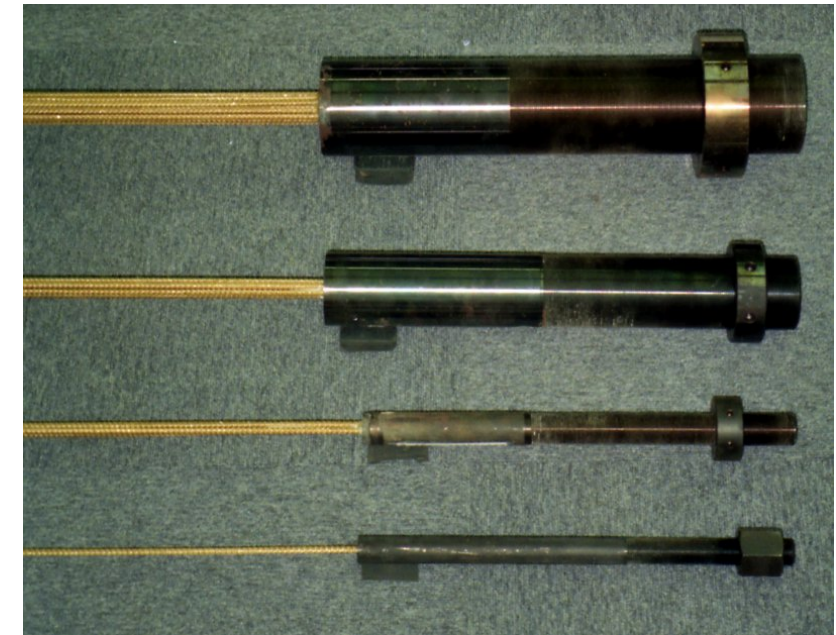
Temporary steel anchorages
